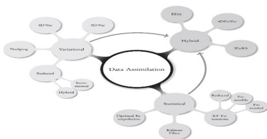
Figure 1. 1. General diagram of current data assimilation methods and techniques for numerical models (M. Asch, M. Bocquet, M. Nodet, 2017)
